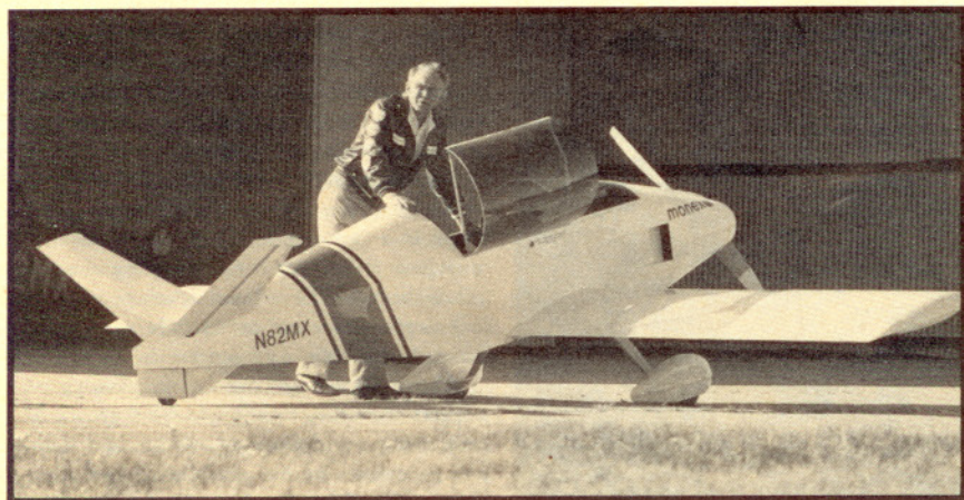
"Dad" Monnett, father of designer John Jr., and the prototype of the latest Monnett design—the Monex. The bonded-wing, single-place airplane features all-aluminum construction.
